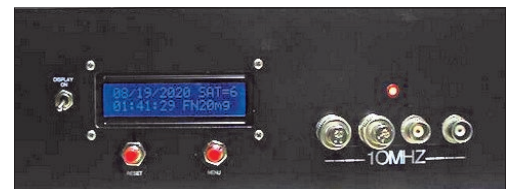
Figure 1 GPS 10 MHz Project with 4 outputs
